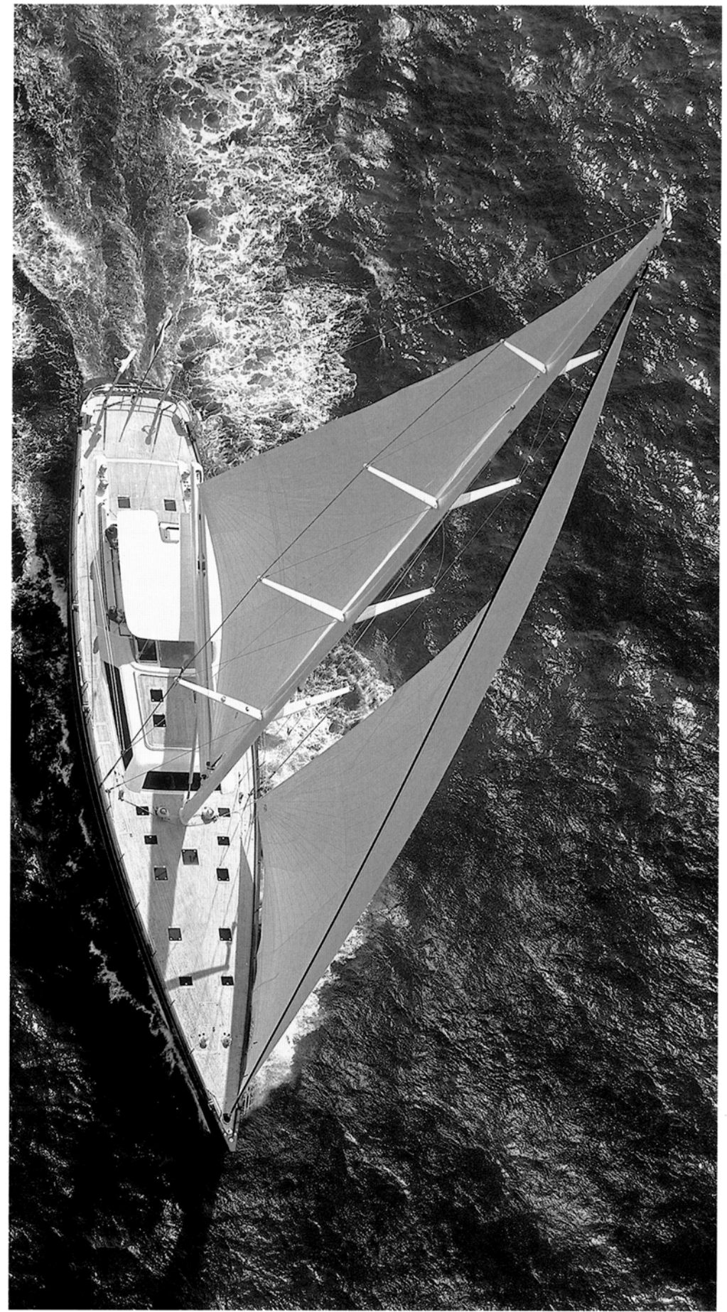
Germán Frers: Swan 112. At 112.27-foot LOA, the Swan 112 is the largest yacht in the Nautor line. These sloops have standardized composite hulls, but otherwise are custom built. The wake gives an idea of the speed this yacht is traveling. With all-power-assisted sail handling it looks like a relaxed and effortless form of transportation. © Nautor/PPL
